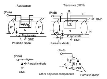
Fig-1 Simplified structure of a Bipolar IC
