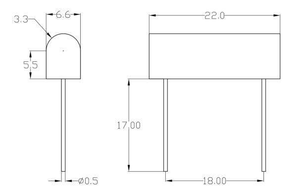
The lead wire is tin plating copper hard wire, the pins haven't positive and negative poles discrimination
