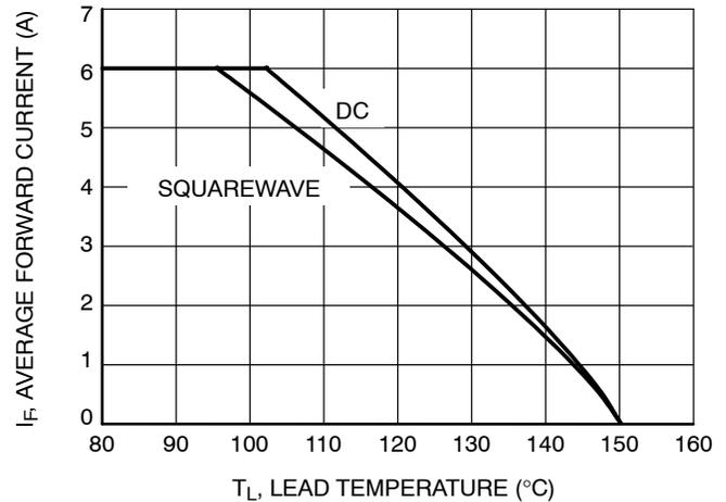
Figure 7. Derating Curve
