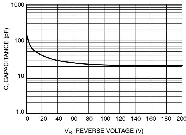
Figure 5. Typical Capacitance
