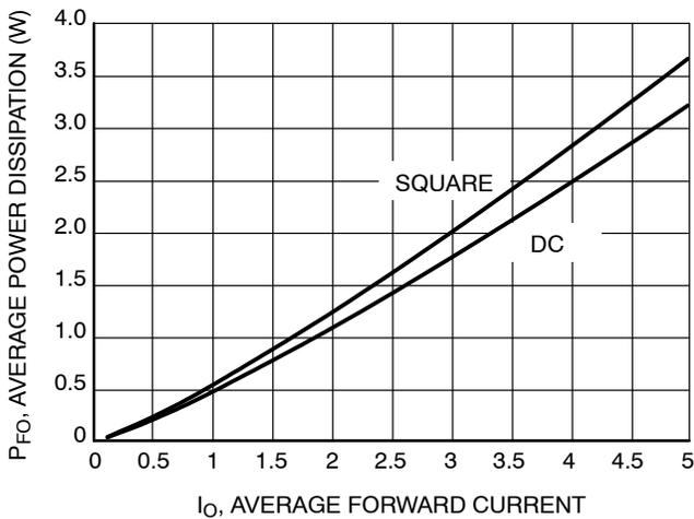
Figure 6. Power Dissipation
