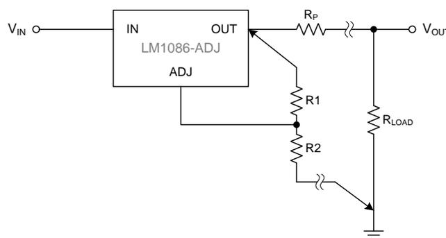
The best load regulation is obtained when the top of the resistor divider R1 is connected directly to the case not to the load. If R1 were connected to the load, the effective resistance between the regulator and the load would be:
