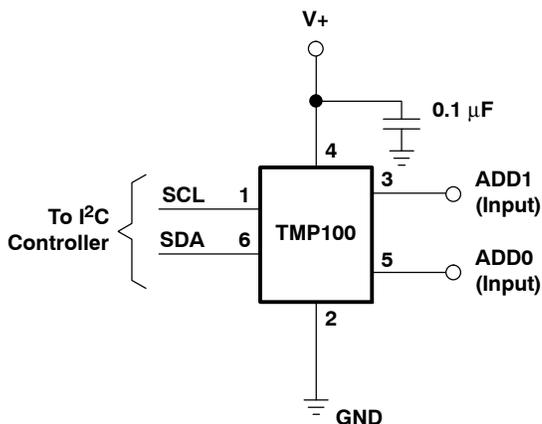
NOTE 2: SCL and SDA require pullup resistors for I<sup>2</sup>C bus applications.
