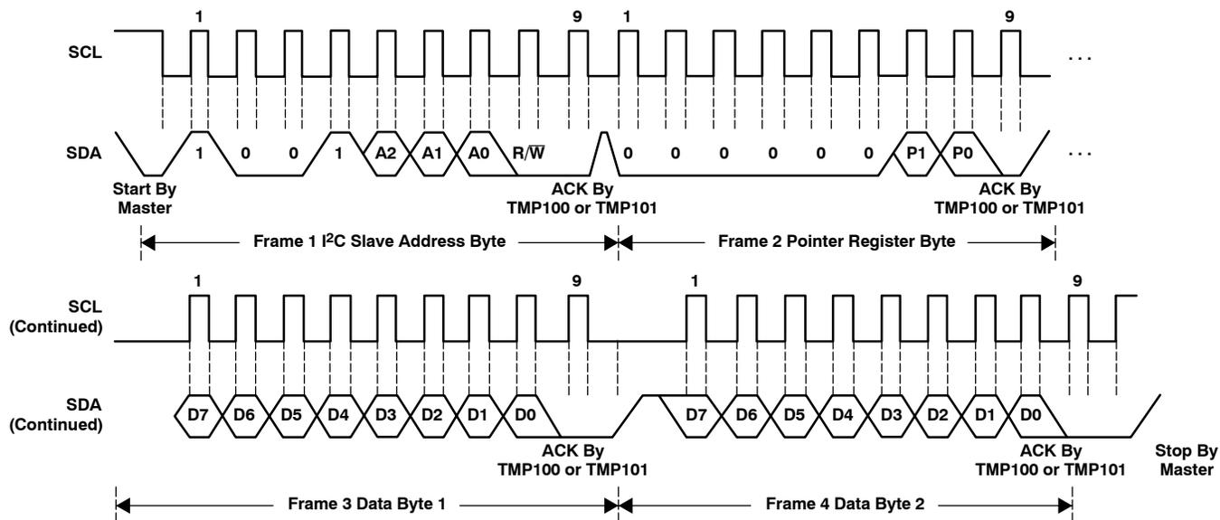
Figure 5. I<sup>2</sup>C Timing Diagram for Write Word Format
