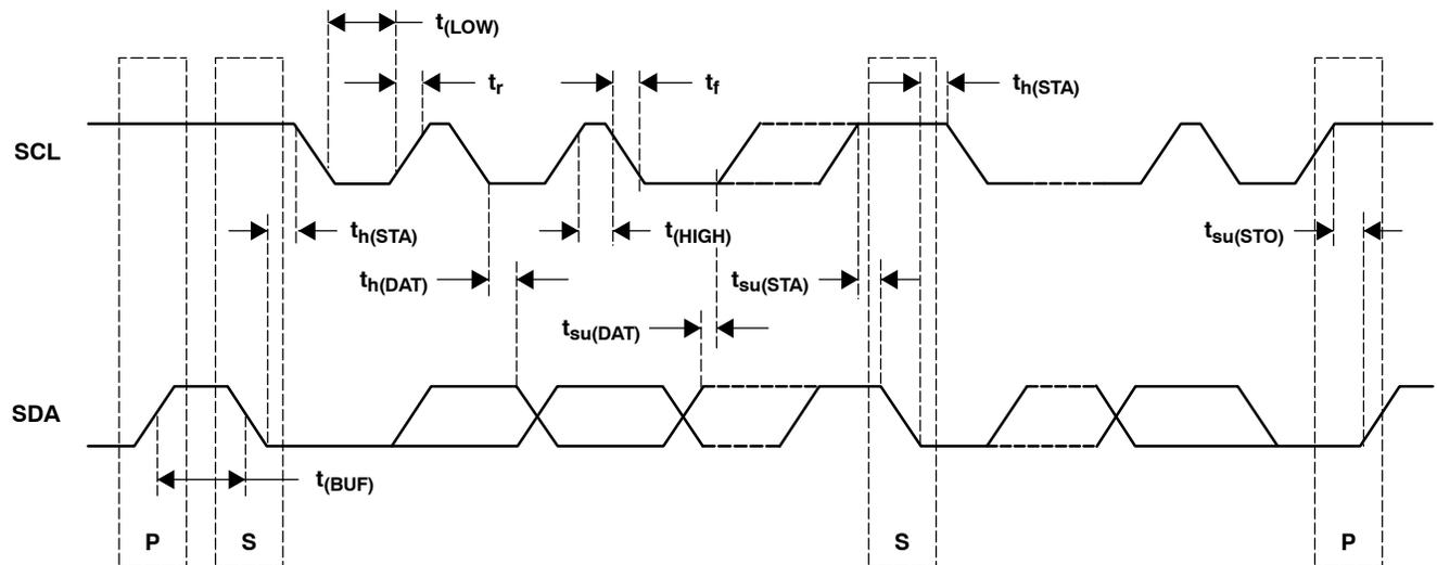
**Figure 4. I<sup>2</sup>C Timing Diagram**
