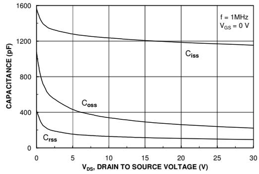
Figure 8. Capacitance Characteristics.
