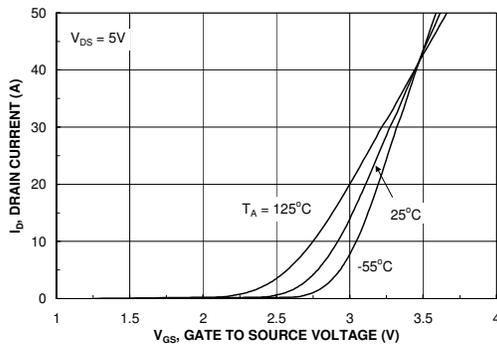
Figure 5. Transfer Characteristics.
