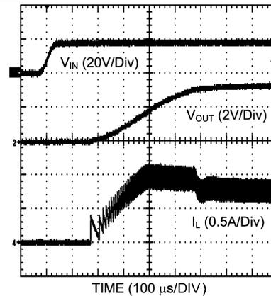
**Figure 12. Power Up ( $V_{OUT} = 3.3\text{ V}$ ,  $0.75\text{ A}$  Loaded)**
