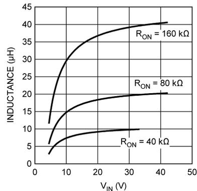
Figure 23. Inductor selection for  $V_{OUT} = 3.3 V$
