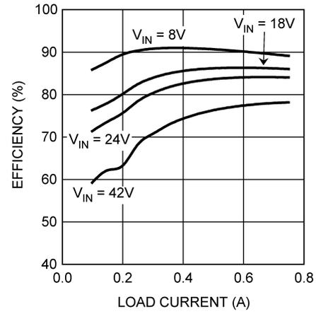
**Figure 8. Efficiency vs Load Current ( $V_{OUT} = 3.3\text{ V}$ )**
