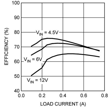
**Figure 10. Efficiency vs Load Current ( $V_{OUT} = 0.6\text{ V}$ )**
