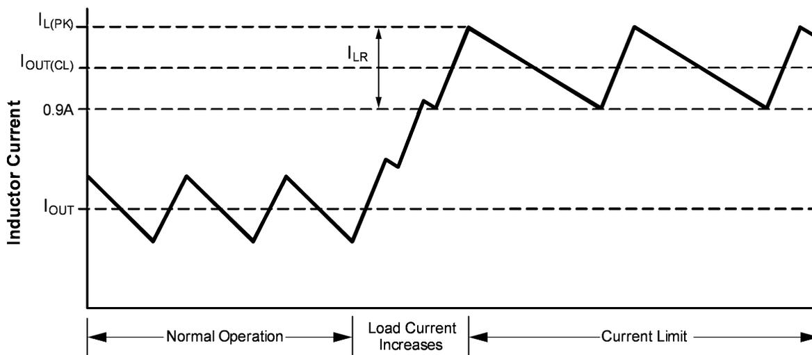
Figure 20. Inductor Current - Current Limit Operation
