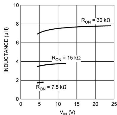
Figure 24. Inductor selection for  $V_{OUT} = 0.6 V$
