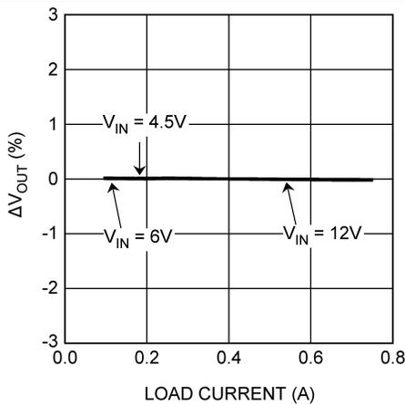
**Figure 11.  $V_{OUT}$  Regulation vs Load Current ( $V_{OUT} = 0.6\text{ V}$ )**
