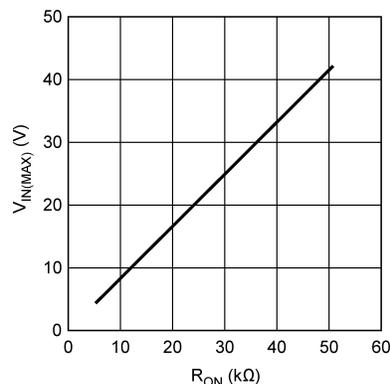
**Figure 22. Maximum V<sub>IN</sub> for selected R<sub>ON</sub>**
