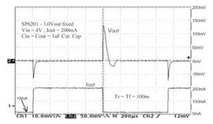
Fig. 34: Load Transient Response, 200mA step, 4V<sub>IN</sub>
