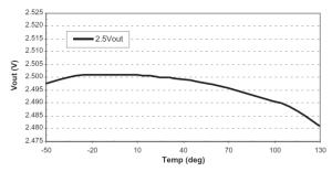
Fig. 16: V<sub>OUT</sub> vs. Temp (adjustable)
