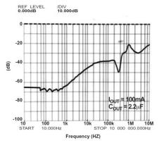
Fig. 41: Power Supply Rejection Ratio
