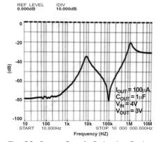
Fig. 38: Power Supply Rejection Ratio
