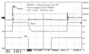
Fig. 30: Inrush Current, Io=100mA
