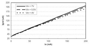
Fig. 11:  $I_{GND}$  vs.  $I_{O}$  (SP6201 fixed 3.0V)
