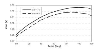
Fig. 13: Vout vs. Temp (fixed 3.3V)
