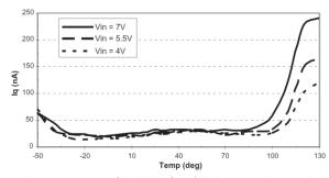
Fig. 9:  $I_q$  vs. Temp (SP6201 fixed 3.0V, EN=0V,  $I_0$ =0uA)
