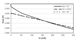
Fig. 19: Load Regulation (SP6201 fixed 3.0V)
