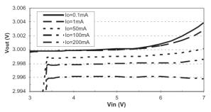
Fig. 18: Line Regulation (SP6201 fixed 3.0V)
