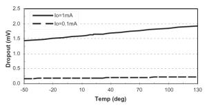
Fig. 6: Dropout vs. Temp (SP6201 fixed 3.0V)
