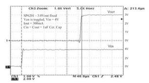
Fig. 24: Turn on time,  $I_0$ =300mA,  $4V_{IN}$
