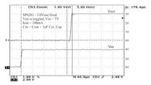
Fig. 25: Turn on time,  $I_0=100mA$ ,  $7V_{IN}$
