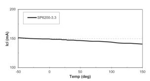
Fig. 21: Current Limit vs. Temp (fixed 3.3V,  $V_{IN}$ =4V)
