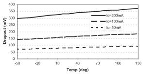
Fig. 5: Dropout vs. Temp (SP6201 fixed 3.0V)
