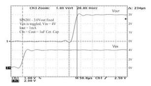
Fig. 22: Turn on time,  $I_0=1mA$ ,  $4V_{IN}$
