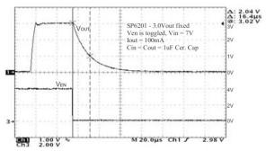
Fig. 29: Turn off time,  $I_{\text{O}} {=}\, 100 \text{mA}, \, 7V_{\text{IN}}$
