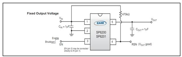
Fig. 1: SP6200 / SP6201 Application Diagram
