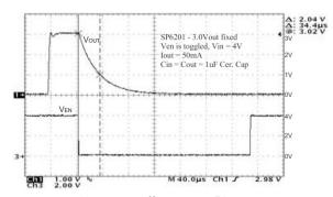
Fig. 27: Turn off time,  $I_0=50mA$ ,  $4V_{IN}$
