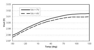
Fig. 12: V<sub>OUT</sub> vs. Temp (fixed 3.0V)
