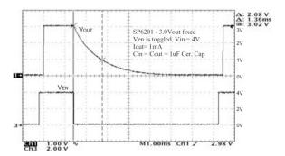
Fig. 26: Turn off time,  $I_0$ =1mA,  $4V_{IN}$
