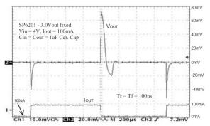
Fig. 32: Load Transient Response, 100mA step, 4V<sub>IN</sub>
