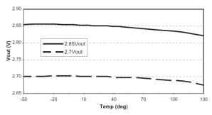
Fig. 14: Vout vs. Temp (adjustable)
