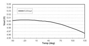
Fig. 17: Vout vs. Temp (adjustable)
