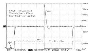
Fig. 35: Load Transient Response, 300mA step, 4VIN
