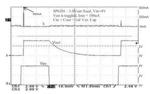
Fig. 31: Inrush Current, I<sub>0</sub>=100μA
