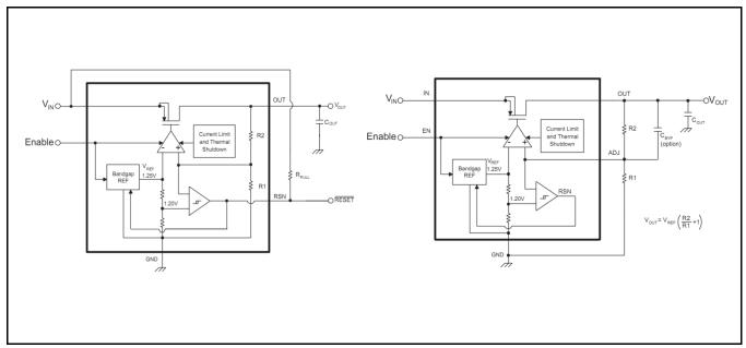
Fig. 2: Fixed Voltage and Adjustable Regulators
