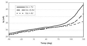
Fig. 8:  $I_q$  vs. Temp (SP6201 fixed 3.0V, EN=Vin,  $I_0$ =0uA)
