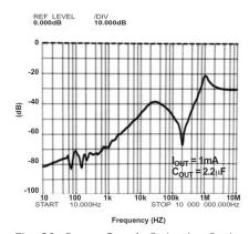
Fig. 39: Power Supply Rejection Ratio
