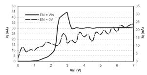
Fig. 7: Iq vs. Vin (fixed 3.0V,  $I_0=0\mu A$ )
