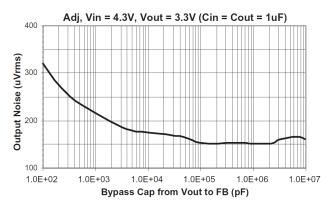
Fig. 42: Noise Performance 10Hz to 100kHz
