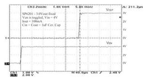
Fig. 23: Turn on time,  $I_0=100mA$ ,  $4V_{IN}$
