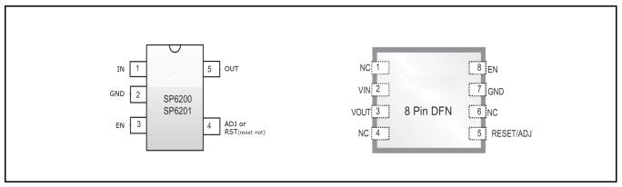
Fig. 3: SP6200 / SP6201 Pin Assignment
