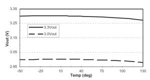
Fig. 15: V<sub>OUT</sub> vs. Temp (adjustable)
