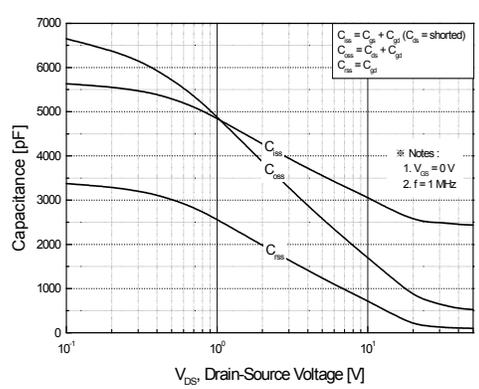
Figure 5. Capacitance Characteristics
