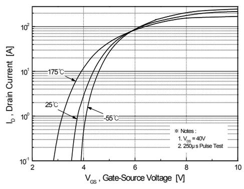
Figure 2. Transfer Characteristics
