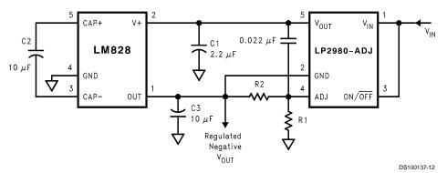
FIGURE 6. Combining LM828 with LP2980 to Make a Negative Adjustable Regulator
