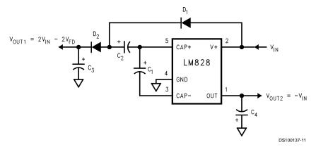
FIGURE 5. Combined Voltage Doubler and Inverter
