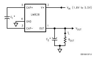
$<sup>^*\</sup>text{C}_1$  and  $\text{C}_2$  are 10  $\mu\text{F}$  capacitors.
