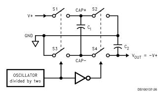
FIGURE 2. Voltage Inverting Principle
