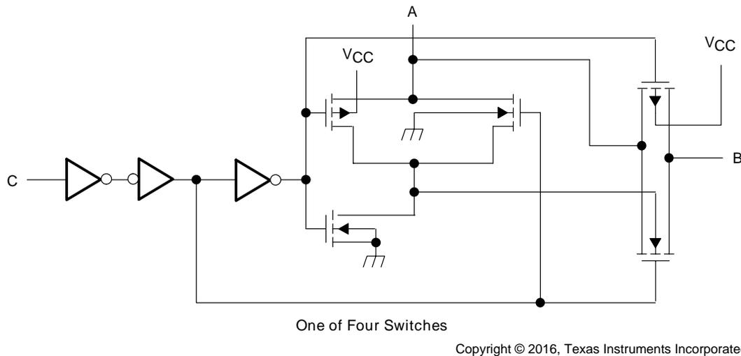
**Figure 13. Logic Diagram, Each Switch (Positive Logic)**
