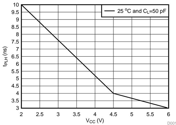
Figure 1. t<sub>PLH</sub> vs V<sub>CC</sub>
