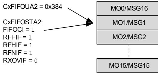
Figure 38-28 illustrates the status of FIFO 2 after one more message is received. Since FIFO 2 is already full, an overflow occurs. The message is discarded and RXOVIF is set. The user address and FIFO index has not changed.
