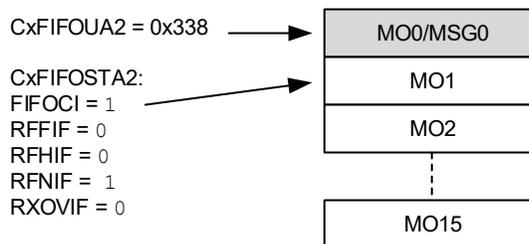
Figure 38-24 illustrates the status of FIFO 2 after MSG0 is read. The user application reads the message from RAM and sets the UINC bit (CxFIFOCON2[8]). The user address increments and points to MO1. The FIFO index is unchanged. The FIFO is empty again. All flags are cleared.
