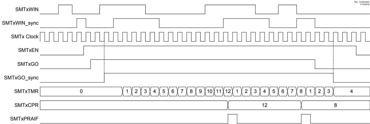
Figure 27-11. Windowed Measurement Mode, Single Acquisition Timing Diagram
