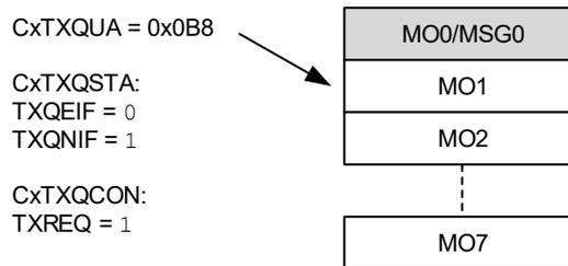
Figure 38-32 illustrates the status of the TXQ after MSG0 is transmitted. The TXQ is empty again. TXQEIF is set and TXREQ is cleared. The user address still points to MO1 because UINC is not set.
