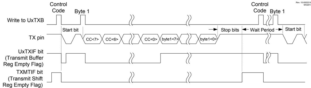
During the communication between two Control Devices, three bytes are required to be transmitted. In this case, the software must write the third byte to UxTXB as soon as UxTXIF goes true and before the output shifter becomes empty. This ensures that the three bytes of the forward frame are transmitted back-to-back without any interruption.
