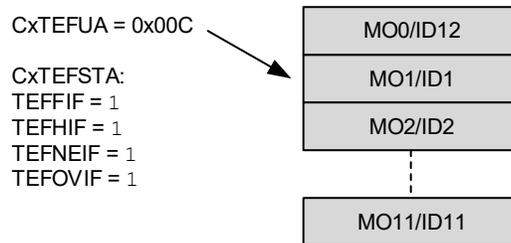
Figure 38-43 illustrates the status of the TEF after the application cleared TEFOVIF and read one more message. TEFFIF is clear because the TEF is not full anymore. The user address points to MO2.
