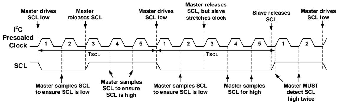
When **FME** is set ( $FME = 1$ ), one SCL period ( $T_{SCL}$ ) is equal to four clock periods of the prescaled **I<sup>2</sup>CxCLK** source. In other words, the prescaled **I<sup>2</sup>CxCLK** source is divided by four. Using the example from above, if the HFINTOSC (4 MHz) clock source is selected, **I<sup>2</sup>CxBAUD** is loaded with a value of '7' and the **FME** bit is set, the actual SCL frequency is 125 kHz (see Equation below).
