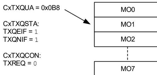
Figure 38-33 illustrates the status of the TXQ after MSG1 is loaded and UINC is set. The user address now points to the next free message object: MO0.
