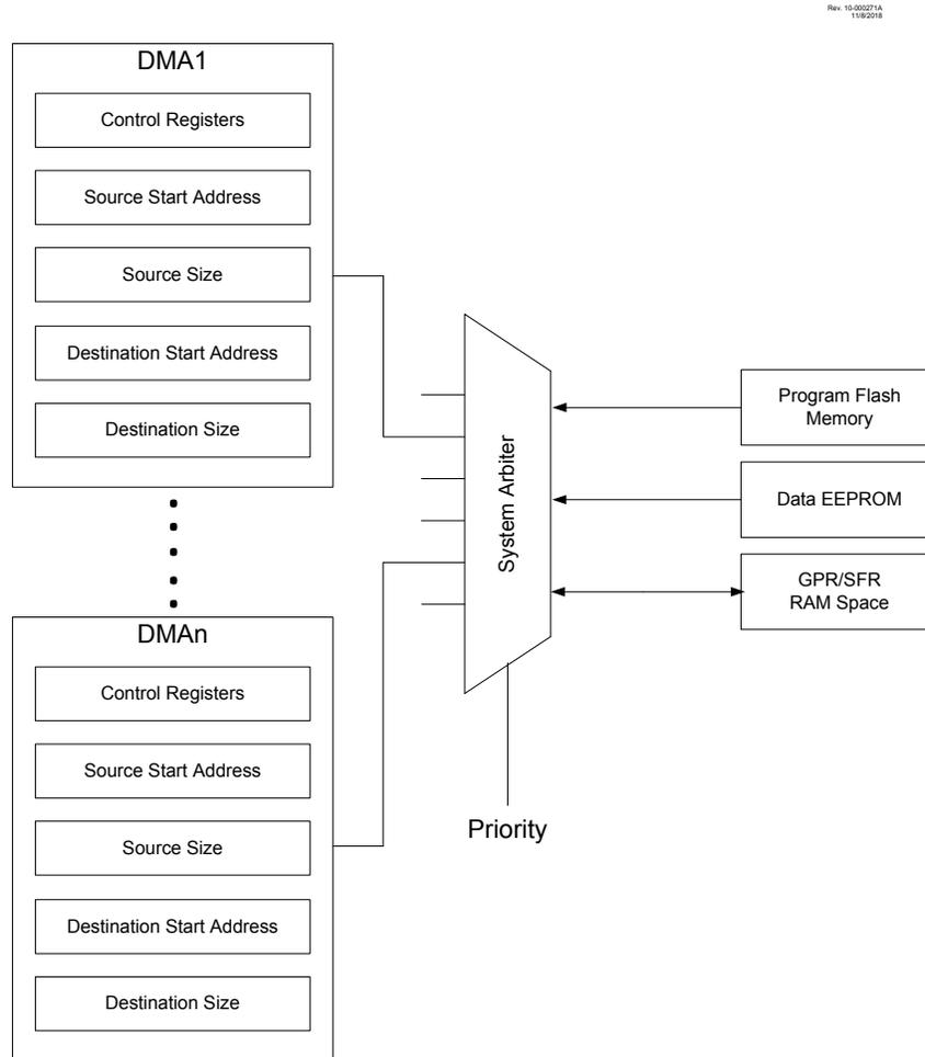
Depending on the priority of the DMA with respect to CPU execution (Refer to section “**Memory Access Scheme**” in the “**PIC18 CPU**” chapter for more information), the DMA Controller can move data through two methods:
