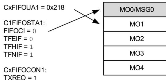
Figure 38-18 illustrates the status of FIFO 1 after MSG0 is transmitted. The FIFO is empty again. TFEIF is set and TXREQ is cleared. FIFOCIX bits now point to MO1 with user address 0x218.
