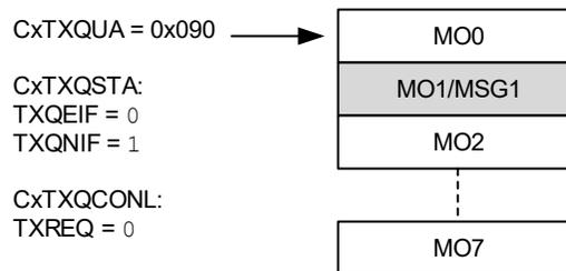
Figure 38-34 illustrates the status of the TXQ after six more messages are loaded: MSG2-MSG7. The user address now points to the last free message object: MO7.
