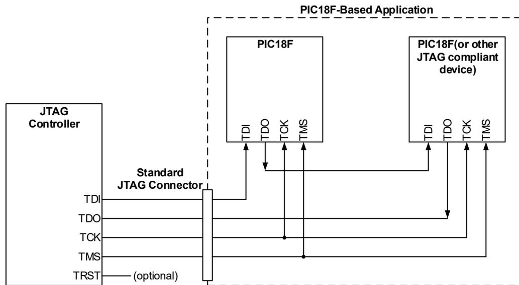
In PIC18-Q83 devices, hardware for the JTAG boundary scan is a Core Independent Peripheral (CIP) with additional integrated logic in all I/O ports. A logical block diagram of the JTAG module is shown in Figure 39-2. It consists of the following key elements:
