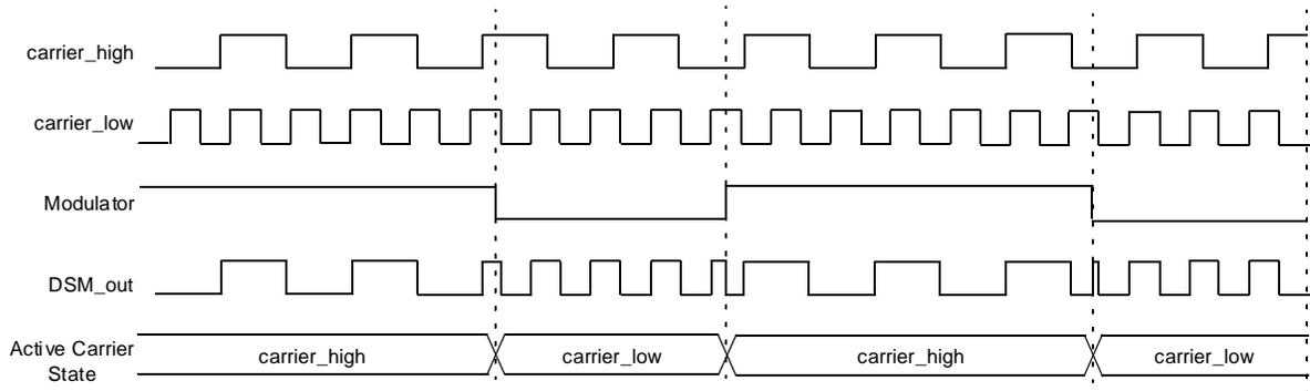
Figure 34-4. Carrier High Synchronization (CHSYNC = 1, CLSYNC = 0)
