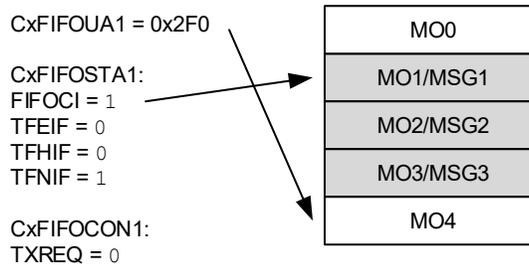
Figure 38-20 illustrates the status of FIFO 1 after two more messages are loaded: MSG4 and MSG5. CxFIFOUA1 now points to MO1. All status flags are now cleared because the FIFO is full. The user address and the FIFO index now point to MO1. The user application now sets TXREQ to request the transmission of MSG1-MSG5.
