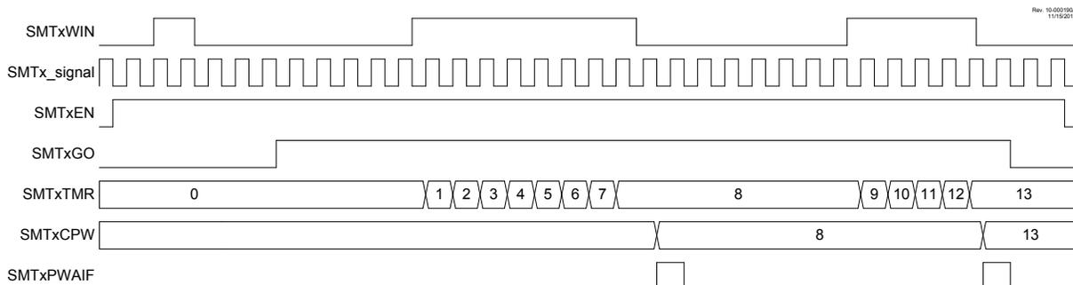
**Figure 27-20. Gated Counter Mode, Single Acquisition Timing Diagram**
