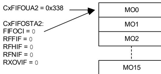
Figure 38-23 illustrates the status of FIFO 2 after the first message (MSG0) is received. MO0 now contains MSG0. The FIFO index now points to MO1. RFNIF is set since the FIFO is not empty anymore.
