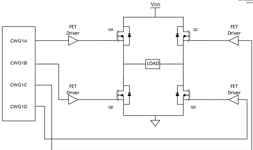
Figure 32-6. Simplified CWG Block Diagram (Forward and Reverse Full-Bridge Modes)
