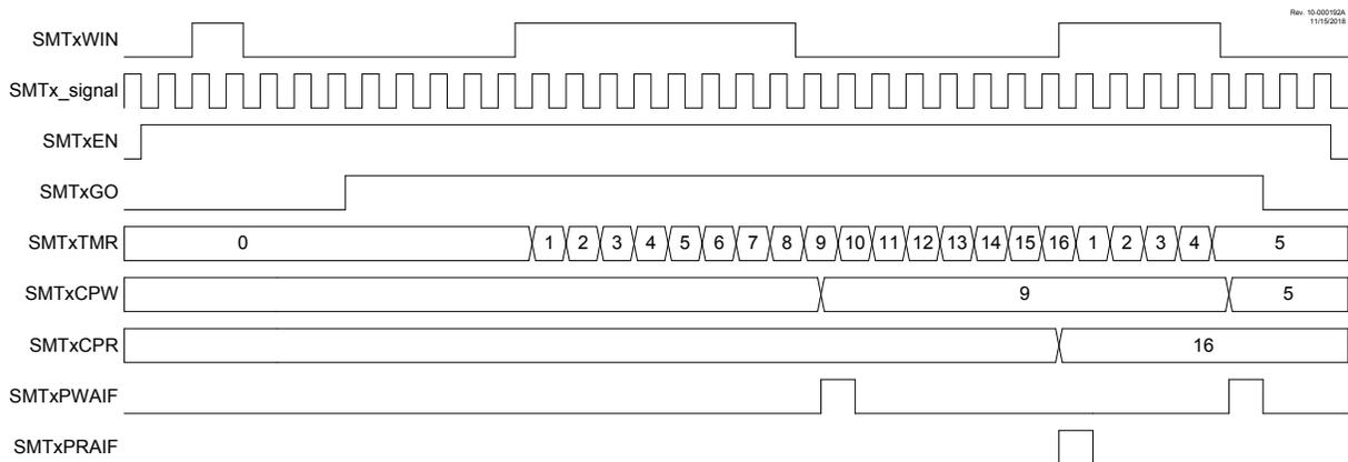
**Figure 27-22. Windowed Counter Mode, Single Acquisition Timing Diagram**
