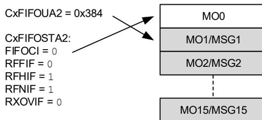
Figure 38-27 illustrates the status of FIFO 2 after one more message is received: MSG16. All status flags are set because the FIFO is full. The user address and the FIFO index point to MO1.
