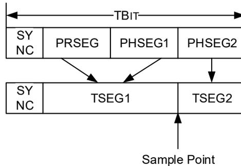
The total number of TQ in a bit time is programmable and can be calculated using [Equation 38-3](#).
