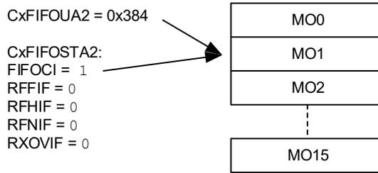
Figure 38-25 illustrates the status of FIFO 2 after eight more messages are received: MSG1-MSG8. The user address still points to MO1. RFNIF and RFHIF are set because the FIFO is now half full. The FIFO index points to MO9.
