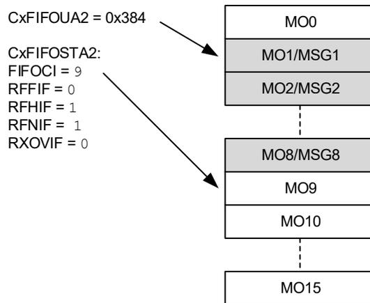
Figure 38-26 illustrates the status of FIFO 2 after ten more messages are received: MSG5-MSG15. The user address still points to MO1. The FIFO index points to MO0. RFNIF and RFHIF are set.
