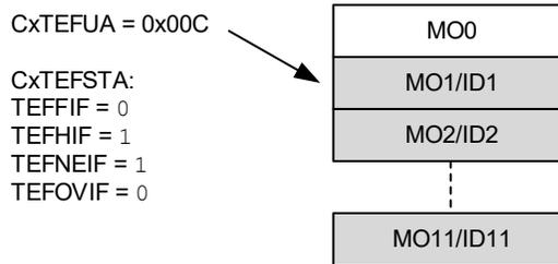
Figure 38-41 illustrates the status of the TEF after one more message is transmitted: MSG12. All status flags are set because the TEF is full. The user address points to MO1.
