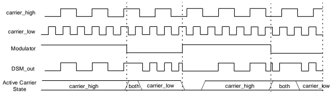
Figure 34-5. Carrier Low Synchronization (CHSYNC = 0, CLSYNC = 1)
