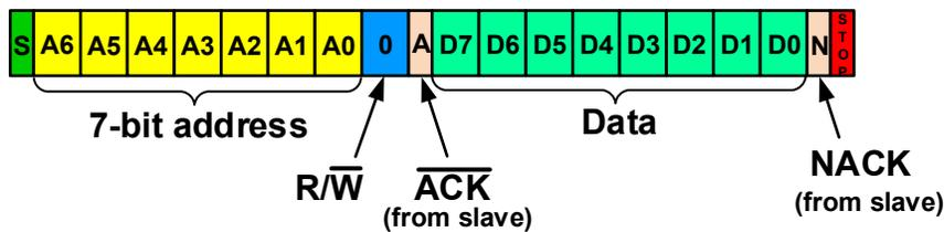
Figure 37-27. 7-Bit Master Write Diagram (to a specific memory/register location)
