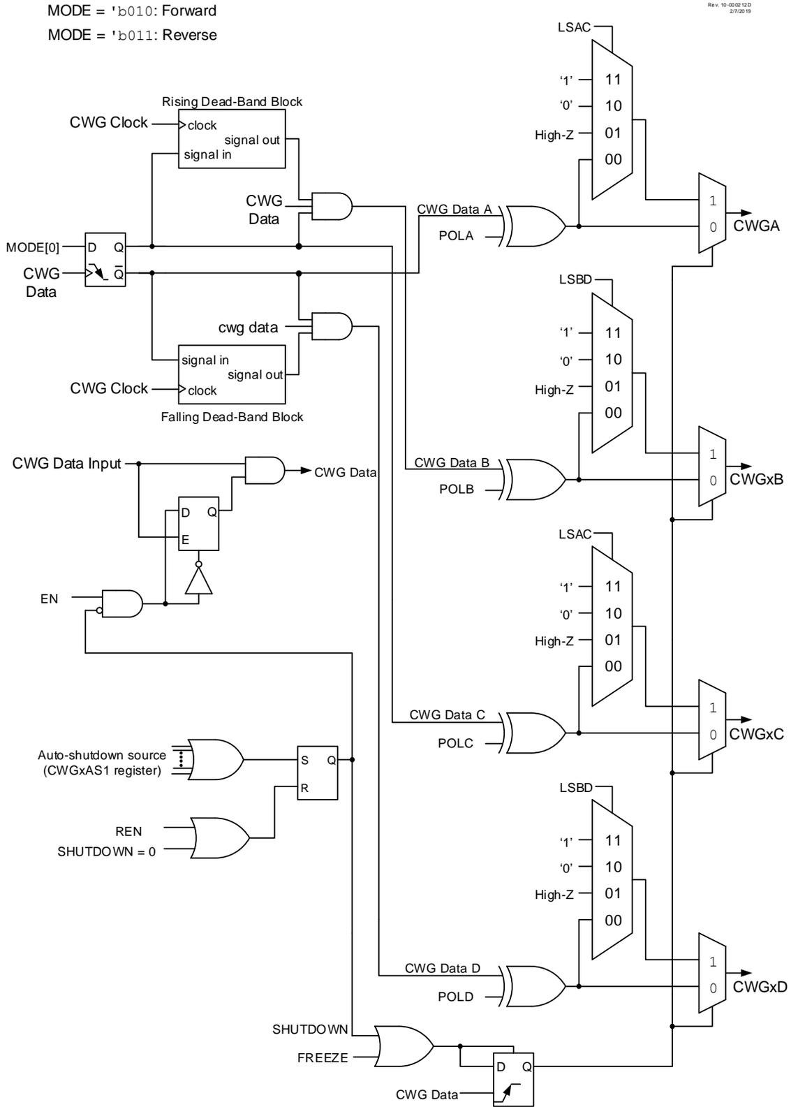
In Forward Full-Bridge mode ( $MODE = 'b010$ ), CWGxA is driven to its Active state, CWGxB and CWGxC are driven to their Inactive state, and CWGxD is modulated by the input signal, as shown in Figure 32-7.
