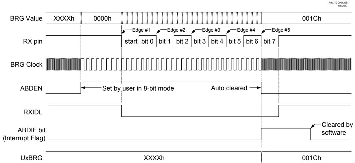
RXIDL indicates that the sync input is active. RXIDL will go low on the first falling edge and go high on the fifth rising edge.
