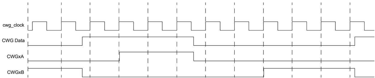
Dead-band is always initiated on the edge of the input source signal. A count of zero indicates that no dead-band is present.
