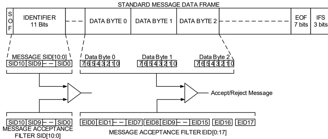
Note: The DeviceNet filtering configuration shown for the EIDx bits is DNCNT[4:0] = 10010.
