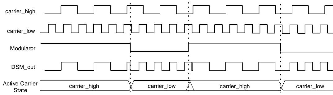
Figure 34-6. Full Synchronization (CHSYNC = 1, CLSYNC = 1)
