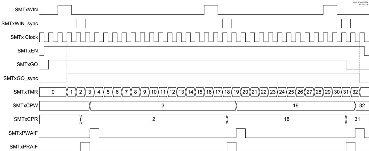
**Figure 27-17. Capture Mode, Single Acquisition Timing Diagram**
