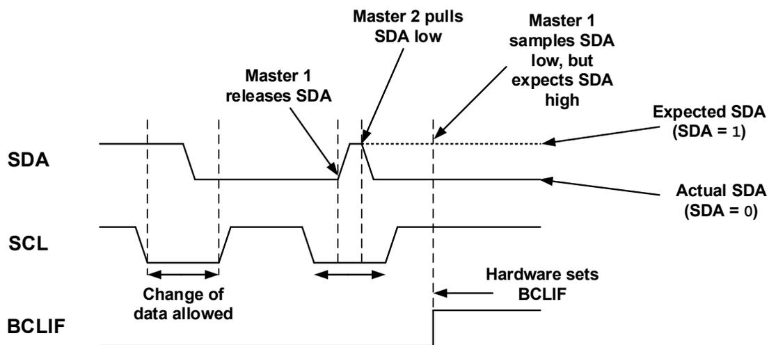
Figure 37-43. Multi-Master Mode Transmission
