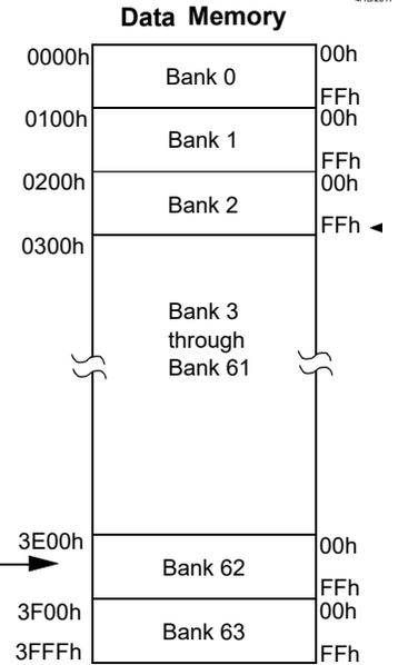
Operations on the FSRs with POSTDEC, POSTINC and PREINC affect the entire register pair; that is, rollovers of the FSRnL register from FFh to 00h carry over to the FSRnH register. On the other hand, results of these operations do not change the value of any flags in the STATUS register (e.g., Z, N, OV, etc.).
