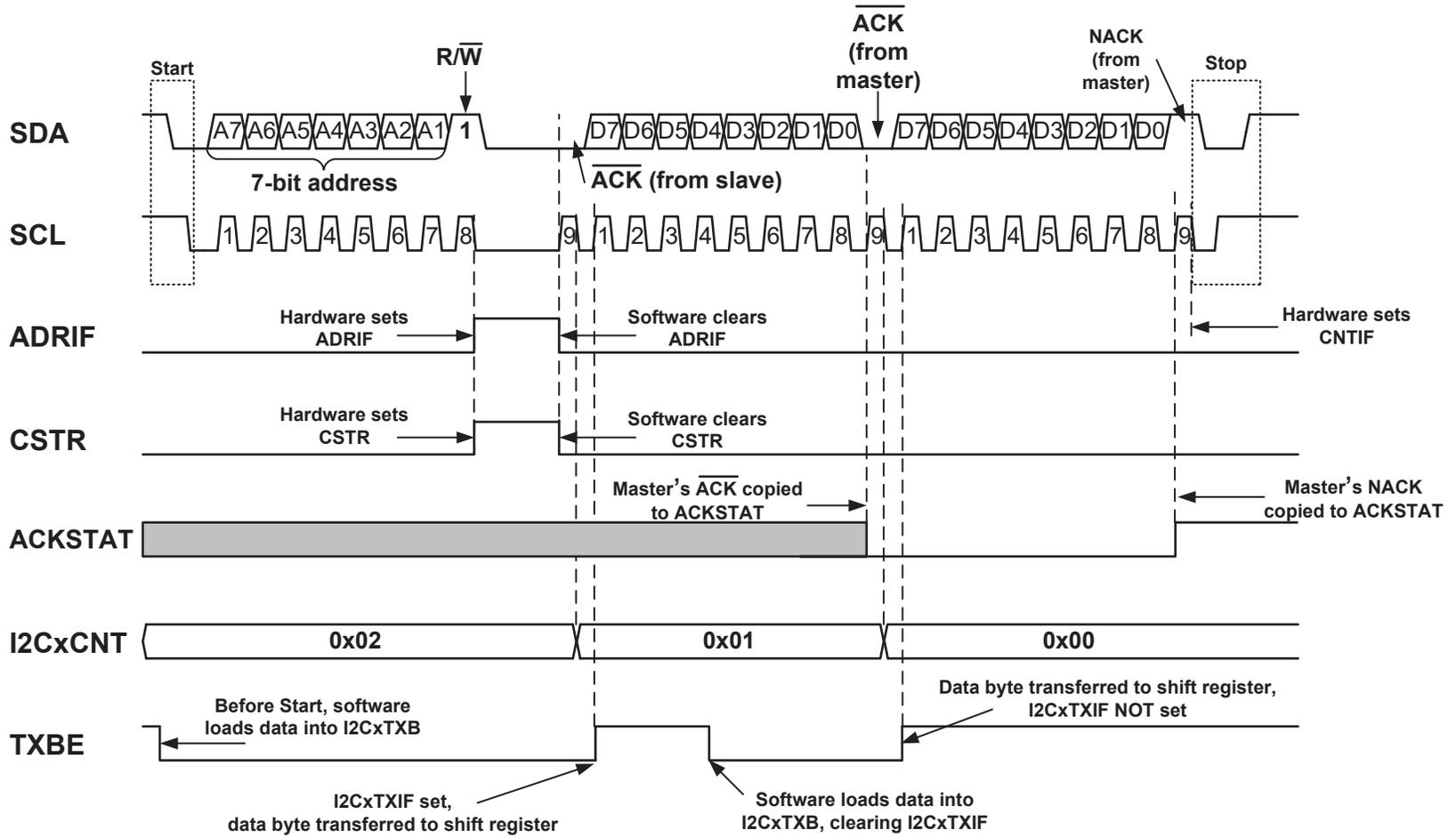
Figure 37-15. 7-Bit Slave Mode Transmission (ACKTIE = 1)
