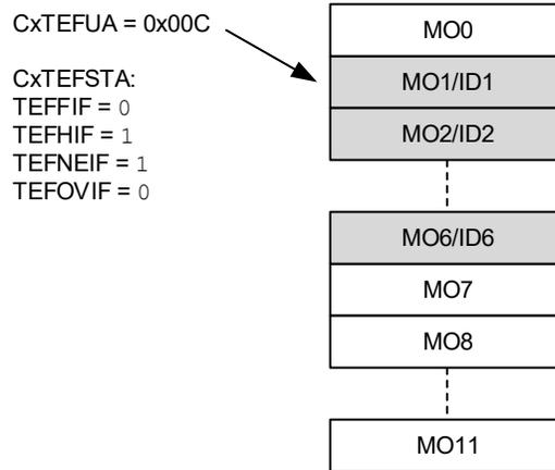
Figure 38-40 illustrates the status of the TEF after five more messages are transmitted: MSG7-MSG11. The user address still points to MO1. TEFNEIF and TEFHIF are set.
