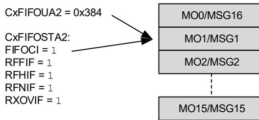
Figure 38-29 illustrates the status of FIFO 2 after the application cleared RXOVIF and read two more messages. RFFIF is clear because the FIFO is not full anymore. The user address points to MO3. The FIFO index has not changed.
