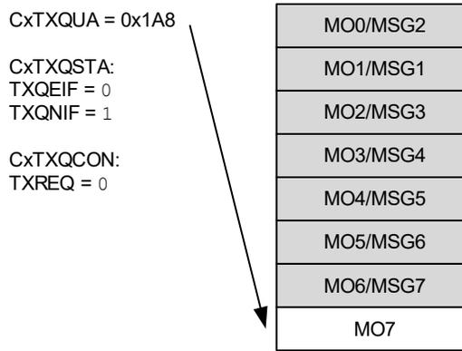
Figure 38-35 illustrates the status of the TXQ after MSG8 is loaded and UINC is set. The TXQ is now full, all flags are cleared. The user address now points to MO0. The user application now sets TXREQ. The messages will be transmitted based on the priority of their IDs.
