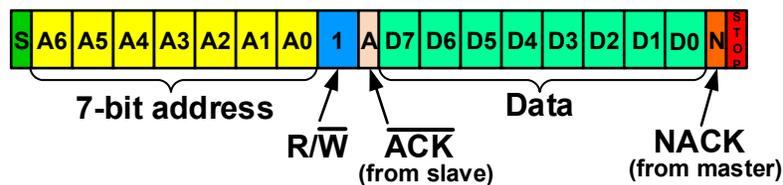
Figure 37-24. 7-Bit Master Read Diagram (from a specific memory/register location)
