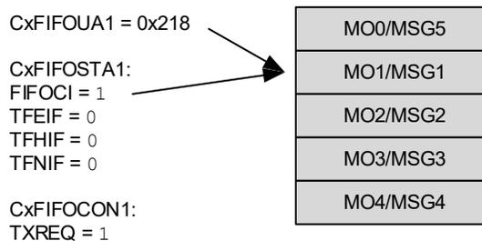
Figure 38-21 illustrates the status of FIFO 1 after MSG1-MSG5 are transmitted. The FIFO is empty again. All status flags are set and TXREQ is cleared. The user address and the FIFO index point to MO1 again.
