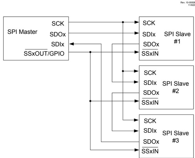
**Figure 36-13. SPI Daisy-Chain Connection With Chained SCK**
