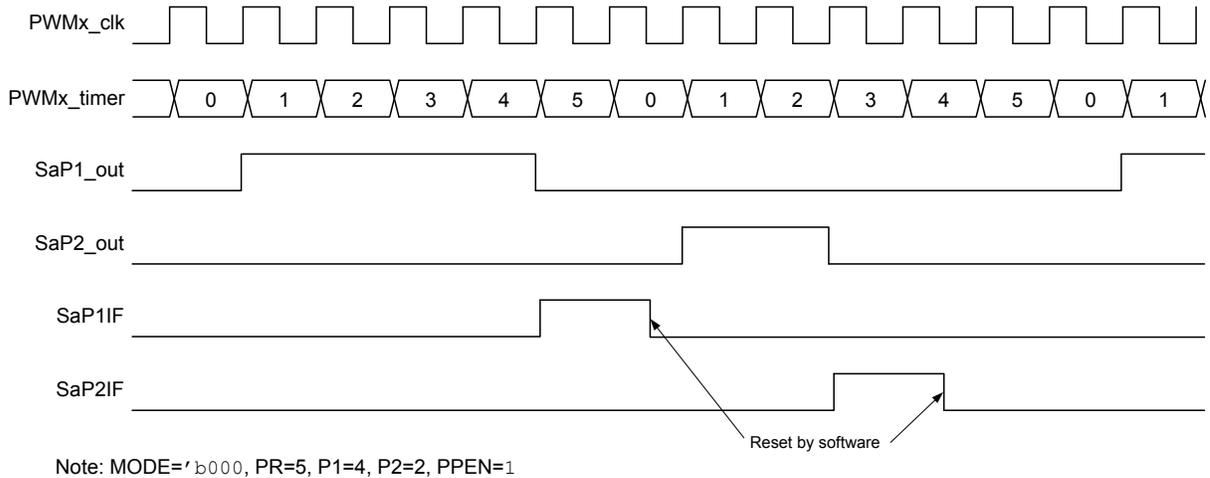
Figure 31-14. Right Aligned Push-Pull Mode Timing Diagram
