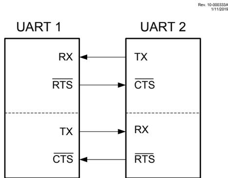
The UART receiving data asserts the  $\overline{\text{RTS}}$  output low when the input FIFO is empty. When a character is received, the  $\overline{\text{RTS}}$  output goes high until the UxRXB is read to free up both FIFO locations.
