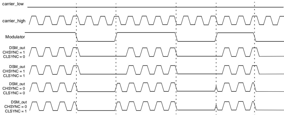
Figure 34-3. No Synchronization (CHSYNC = 0, CLSYNC = 0)
