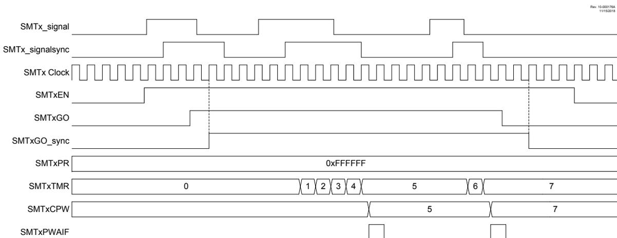
Figure 27-5. Gated Timer Mode, Single Acquisition Timing Diagram
