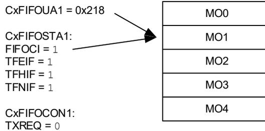
Figure 38-19 illustrates the status of FIFO 1 after three more messages are loaded: MSG1-MSG3. The user address now points to MO4. TFHIF is cleared because the FIFO is now less than half empty.
