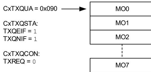
Figure 38-31 illustrates the status of the TXQ after the first message (MSG0) is loaded. MO0 now contains MSG0. The user application sets the UINC bit, which causes the FIFO head to advance. The user address now points to MO1. TXQEIF is cleared, since the queue is not empty anymore. The user application now sets TXREQ to request the transmission of MSG0.
