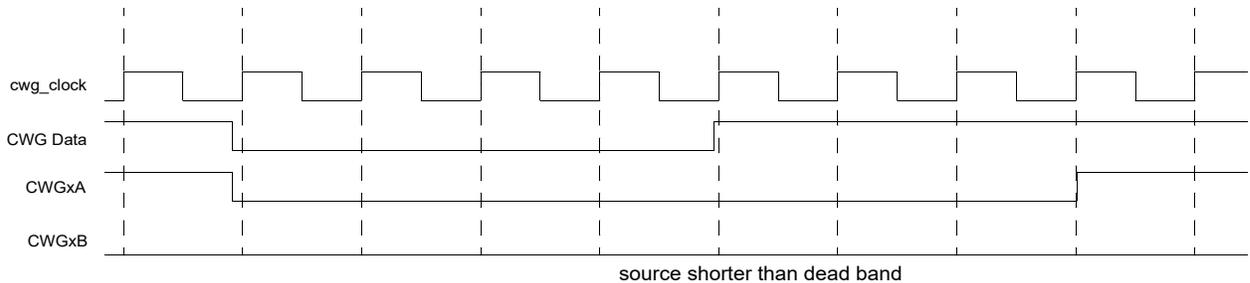
The CWGxDBF register value is double-buffered. When EN = 0, the buffer is loaded when CWGxDBF is written. When EN = 1, then the buffer will be loaded at the rising edge following the first falling edge of the data input after the LD is set.
