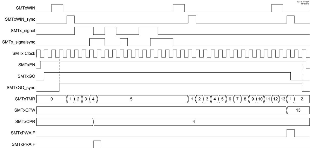
**Figure 27-15. Time-of-Flight Mode, Single Acquisition Timing Diagram**
