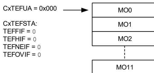
Figure 38-37 shows the status of the TEF after the first transmit message is stored. MO0 contains ID0, the ID of MSG0. TEFNEIF is set since the TEF is not empty. The user address points to MO0.
