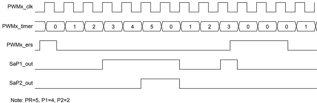
**Figure 31-16. Left Aligned Mode with ERSNOW = 0**
