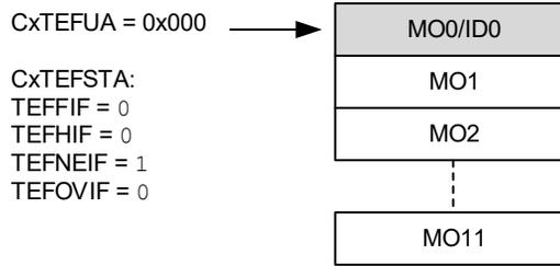
Figure 38-38 illustrates the status of the TEF after ID0 is read. The user application reads the ID from RAM and sets the UINC bit (C1TEFCONL[8]). The user address increments and points to MO1. The TEF is empty again. All flags are cleared.
