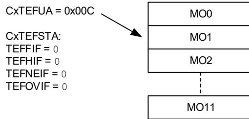
Figure 38-39 illustrates the status of the TEF after six more messages are transmitted: MSG1-MSG6. The user address points to MO1. TEFNEIF and TEFHIF are set because the TEF is now half full.
