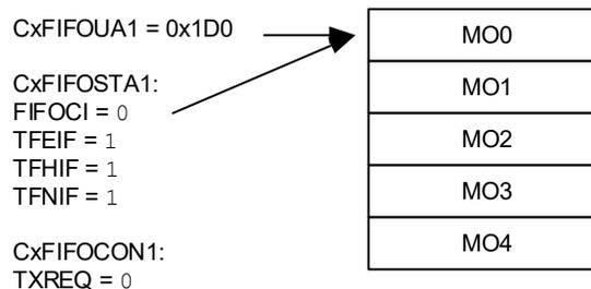
[Figure 38-17](#) illustrates the status of FIFO 1 after the first message (MSG0) is loaded. MO0 now contains MSG0. The user application sets the UINC bit (CxFIFOCON1[8]), which causes the FIFO head to advance. The user address now points to MO1. TFEIF is cleared since the FIFO is no longer empty. The user application now sets TXREQ to request the transmission of MSG0.
