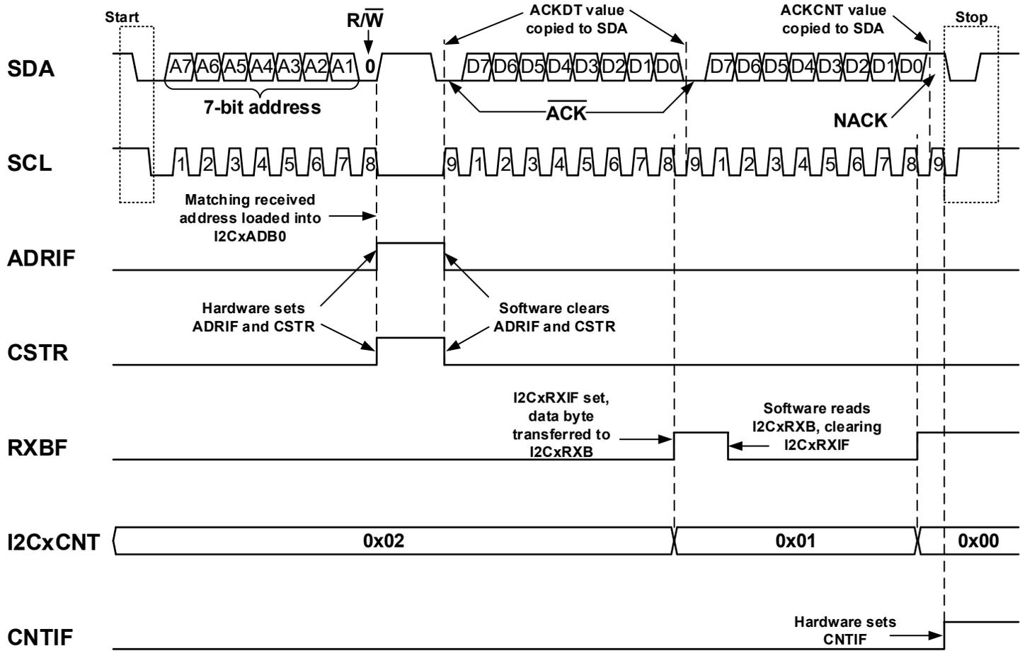
Figure 37-18. 7-Bit Slave Mode Reception (ACKTIE = 1)
