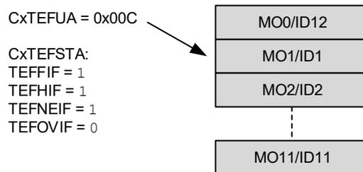
Figure 38-42 illustrates the status of the TEF after one more message is transmitted. Since the TEF is already full, an overflow occurs. The ID is discarded and TEFOVIF is set. The user address remains unchanged.
