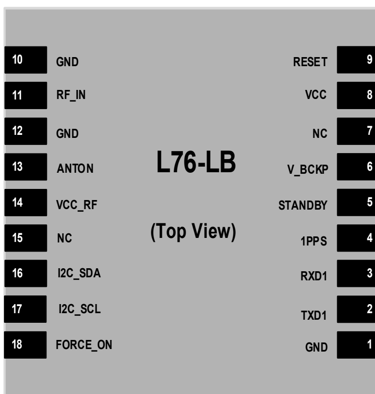
Figure 2: Pin Assignment
