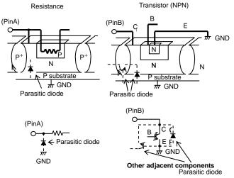
Fig.1 Simplified structure of a Bipolar IC
