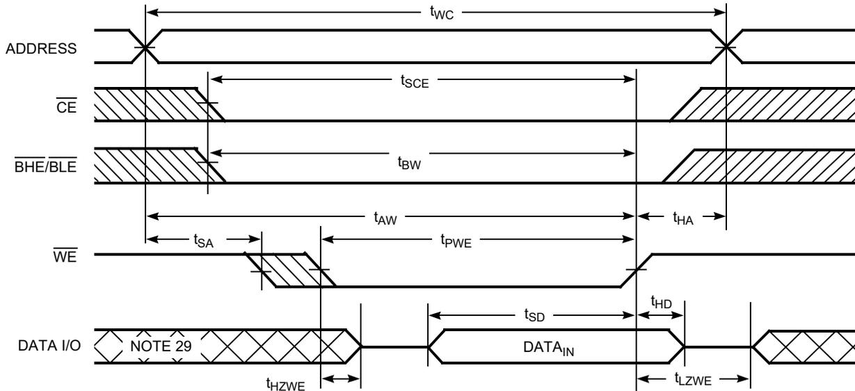
Figure 9. Write Cycle 4:  $\overline{BHE}/\overline{BLE}$  Controlled,  $\overline{OE}$  LOW<sup>[27, 28]</sup>
