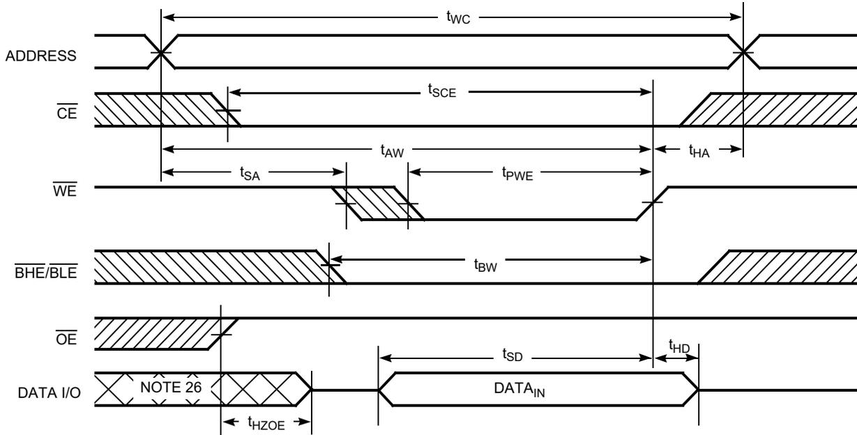
Figure 7. Write Cycle 2:  $\overline{CE}$  Controlled<sup>[23, 24, 25]</sup>
