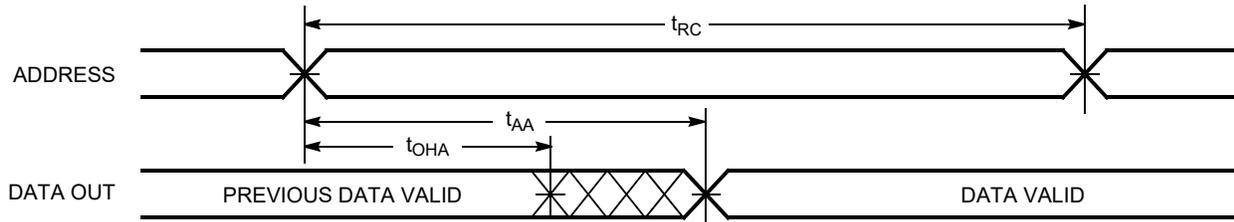
Figure 5. Read Cycle No. 2:  $\overline{OE}$  Controlled<sup>[21, 22]</sup>
