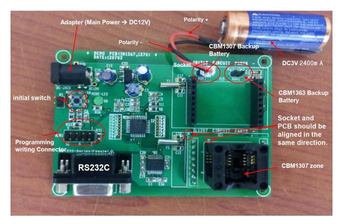
Fig 2 Top view of test fixture
