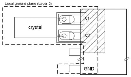
Figure 5. Recommended layout for crystal.
