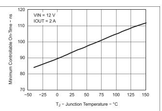
Figure 14. Minimum Controllable On-Time vs Temperature
