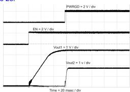
Figure 26. Sequential Start-Up Sequence
