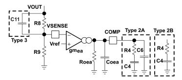
Figure 23. Types of Frequency Compensation
