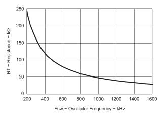
Figure 24. RT Set Resistor vs Switching Frequency
