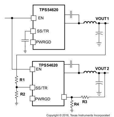
Figure 30. Ratiometric and Simultaneous Start-Up Sequence
