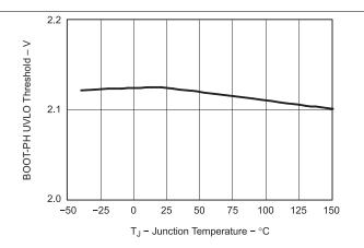
Figure 16. BOOT-PH UVLO Threshold vs Temperature
