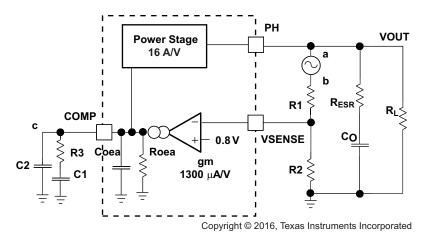
Figure 20. Small Signal Model for Loop Response
