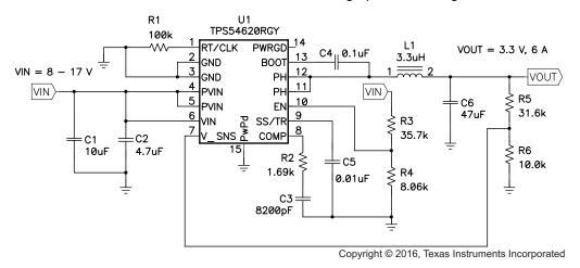
Figure 34. Typical Application Circuit
