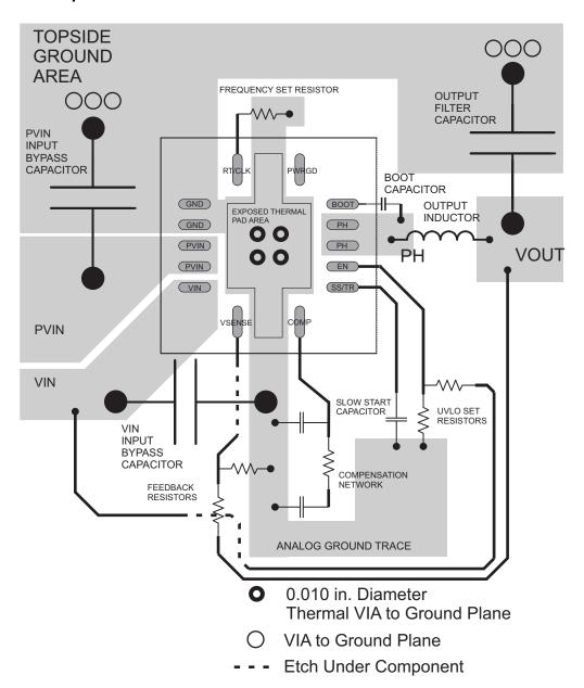
Figure 55. PCB Layout
