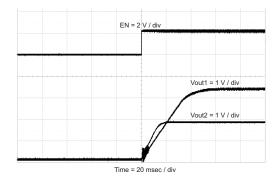
Figure 31. Ratiometric Start-Up With Vout1 Leading Figure 32. Ratiometric Start-Up With Vout2 Leading Vout1
