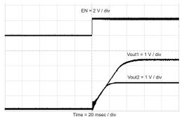
Figure 33. Simultaneous Start-Up
