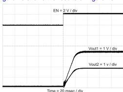
Figure 28. Ratiometric Start-Up Sequence
