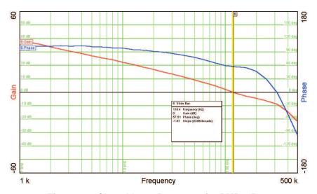
Figure 36. Closed-Loop Response for PMP4854-2
