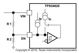
Figure 17. Adjustable VIN Undervoltage Lockout
