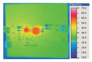
Figure 57. Thermal Signature of TPS54620EVM-374 Operating at  $V_{IN}$  = 12 V,  $V_{OUT}$  = 3.3 V, 6 A,  $T_A$  = Room Temperature
