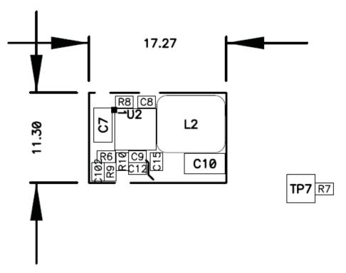
Figure 56. Ultra-Small PCB Layout Using TPS54620 (PMP4854-2)
