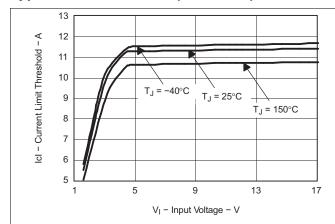
Figure 13. High-Side Current Limit Threshold vs Input Voltage
