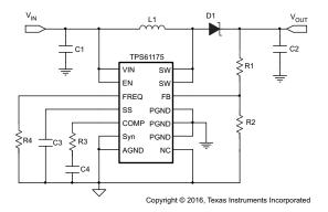
Figure 8. Boost Converter Configuration
