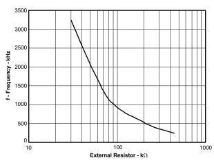
Figure 7. Switching Frequency vs External Resistor
