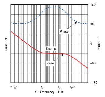
Figure 11. Bode Plot of Feedback Resistors and Compensated Amplifier Gain and Phase
