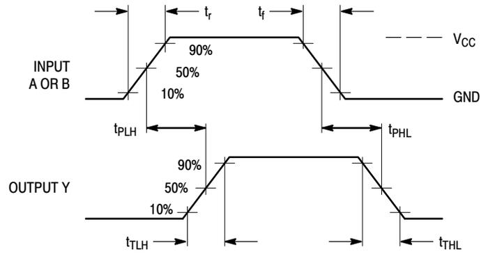
Figure 1. Switching Waveforms
