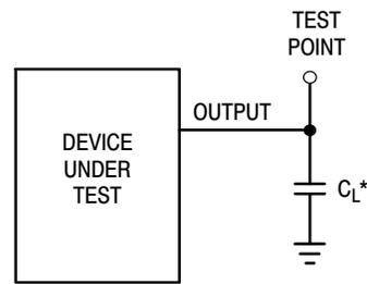
\*Includes all probe and jig capacitance
