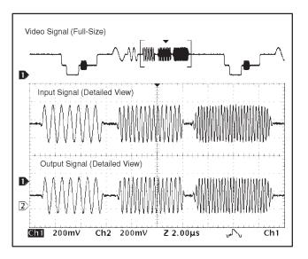
Figure 3. Multiburst (CCIR 18) Test Pattern (PAL)
