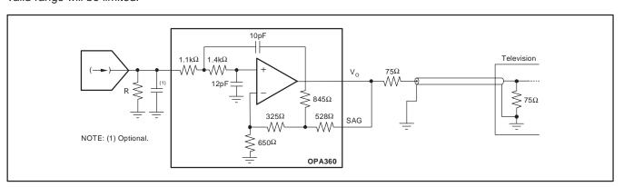
Figure 1. Filter Structure of OPA360
