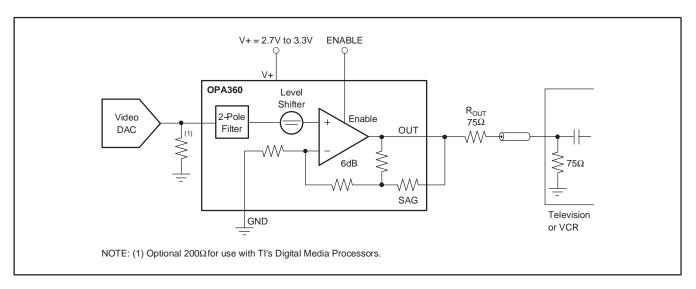
Figure 15. DC-Coupled Input/DC-Coupled Output
