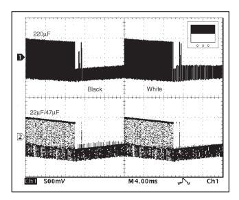
Figure 10. Standard Video Circuit with 220μF Capacitor (top trace) vs OPA360 with 22μF and 47μF Capacitors
