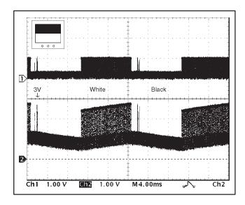
Figure 12. Output Swing with 47μF on 3V Supply
