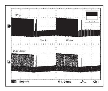
Figure 11. 220μF Standard Video Circuit (top trace) vs OPA360 with 22μF and 67μF Capacitors
