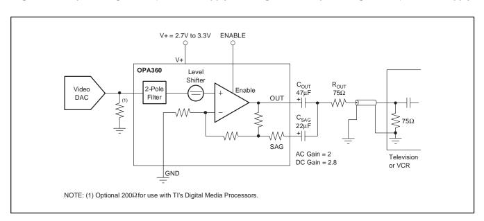
Figure 14. DC-Coupled Input/AC-Coupled Output
