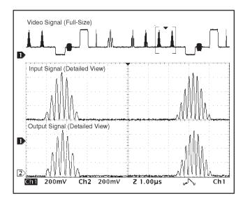
Figure 4. Multipulse Test Pattern (PAL)
