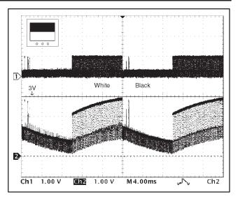
Figure 7. Output Swing with 33µF on 3V Supply
