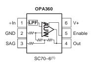
(1) Pin 1 of the SC70-6 is determined by orienting the package marking as indicated in the diagram.
