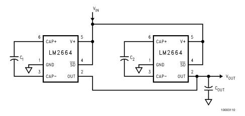
FIGURE 3. Lowering Output Resistance by Paralleling Devices
