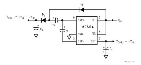
FIGURE 5. Combined Voltage Doubler and Inverter
