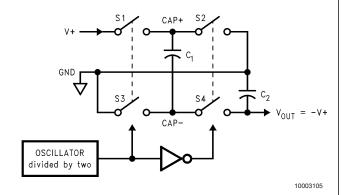
FIGURE 2. Voltage Inverting Principle
