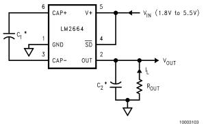
$^*\text{C}_1$  and  $\text{C}_2$  are 3.3  $\mu\text{F},$  SC series OS-CON capacitors.
