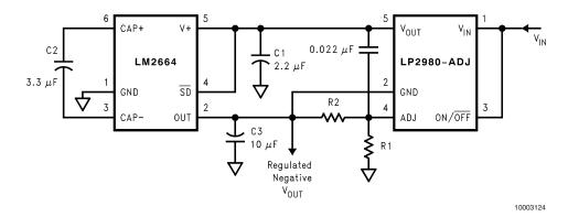
FIGURE 6. Combining LM2664 with LP2980 to Make a Negative Adjustable Regulator
