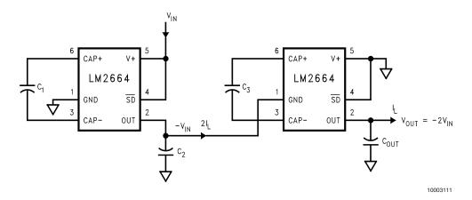
FIGURE 4. Increasing Output Voltage by Cascading Devices
